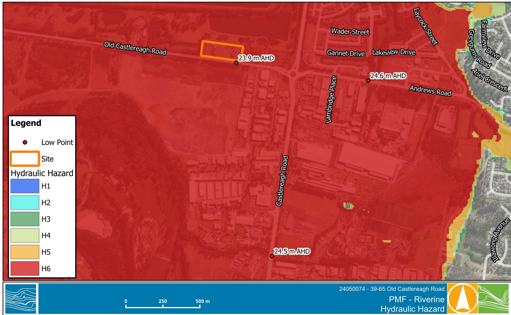
Figure 2-5 Hydraulic hazard in the riverine PMF
